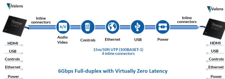
HDBaseT Automotive is a derivative of HDBaseT, a mature, proven and standardized technology for the transmission of ultra-high-definition audio & video, controls, Ethernet, USB and power in the consumer electronics and professional audiovisual markets. Millions of chips have been deployed worldwide, empowering thousands of HDBaseT products.
