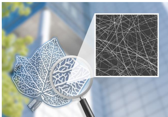
Figure: OPVIUS' free-form OPV module based on a TPK transparent, conductive foil substrate coated with Cambrios ClearOhm ® silver nanowires
