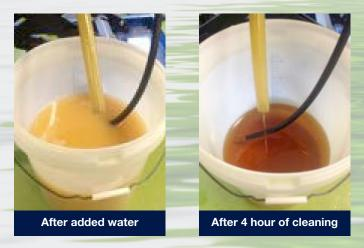
After 4 hours of cleaning, the oil is better than new oil and the reduction of water in the oil after the test is 99.3%. In addition, the reduction of particles after the test is 80.2%.
