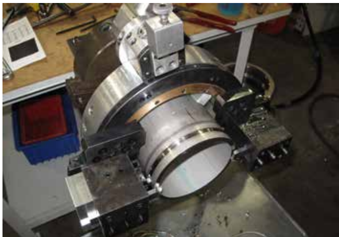
This custom configured grooving machine was designed to provide precision end grooves to match couplings to construct a military, rapid-deployment, fuel pipeline during Operation Desert Storm.
