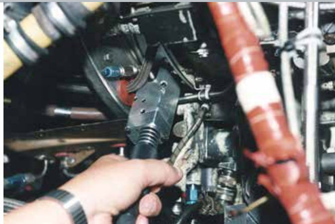
Our compact (no debris) roller-wheel tubing cutter was designed to perform precision tube severing in tight spaces. This machine is included in most front-line military aircraft maintenance equipment.
