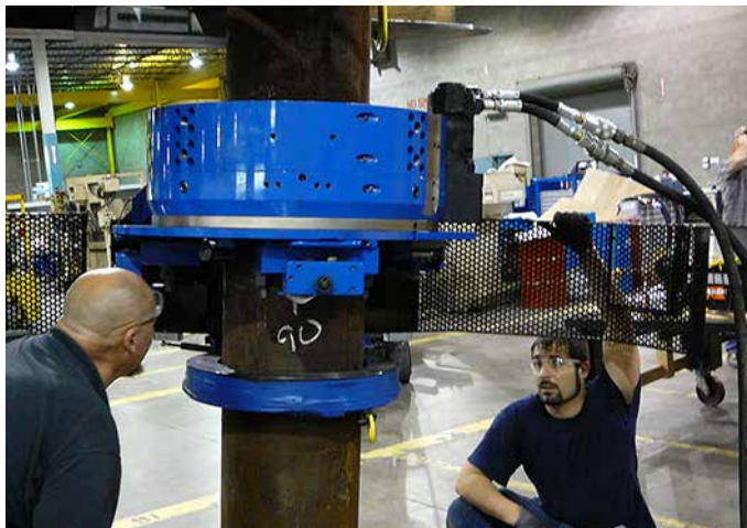
This custom engineered and built automatic-mounting High Speed Severing System was designed to rapidly cut-out defective welds for re-welding in an offshore J-Lay pipeline barge production role.
