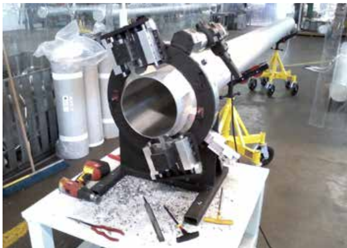
This RBL clamshell has been custom configured with a bench stand, electric drive, and features a full support clamping system and spring actuated cutting heads - both to correct out-of-round issues.
