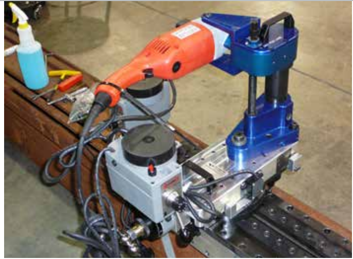
The track milling system above was designed utilizing our Model 424 Keyway Cutter. The machine is guided by a custom track that is temporarily welded in place to provide stability and precision results.
