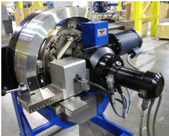
This remote-controlled CNC Machining System with control computer was designed as a fully custom solution for extremely accurate 3-axis cutting in the hazardous environment of a Nuclear Power Plant.
