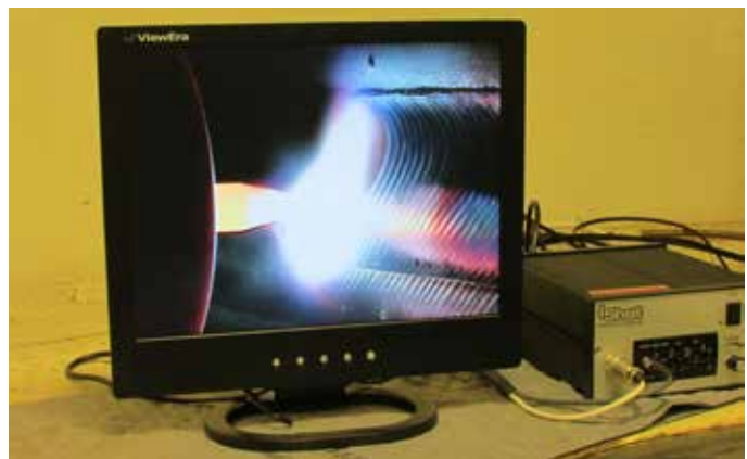
The introduction of electronics to our custom engineered equipment solutions has become much more prevalent such as this integral video system being used to monitor a critical welding operation.
