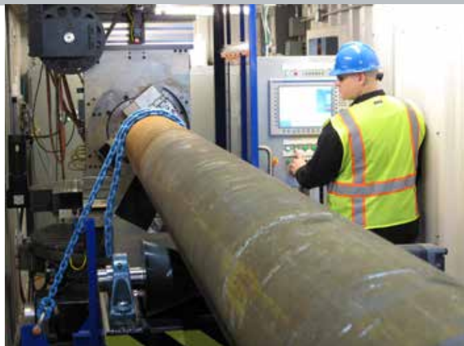
A custom deep counterboring system was needed for a major onshore pipe fabrication project. Our custom system was deployed with a completely custom built pipe rack featuring maximum safety.
