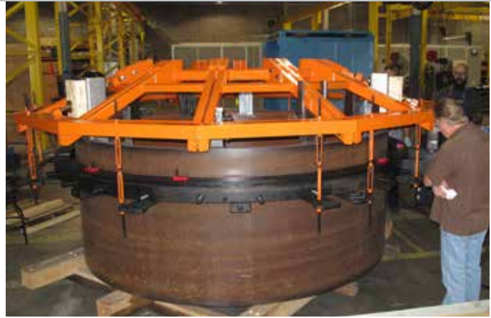
A fully adjustable machine support was created to carry the weight and forces of operating a custom engineered 160" lathe. The lathe first performed precision cutting and then a weld head was then mounted to the lathe's rotating ring to perform accurate fill welding of the machined sections.
