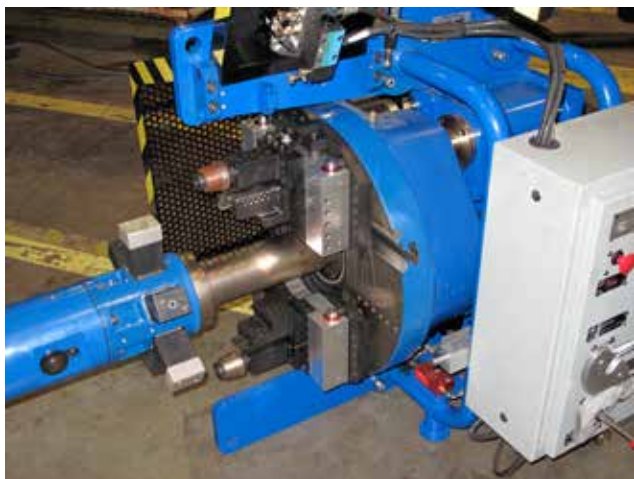
Designed to eliminate weld prep bevel inconsistencies that occur from out-of-round conditions, this pipe facing machine is fitted with custom-built OD tracking tool holders for uniform bevel profiles.
