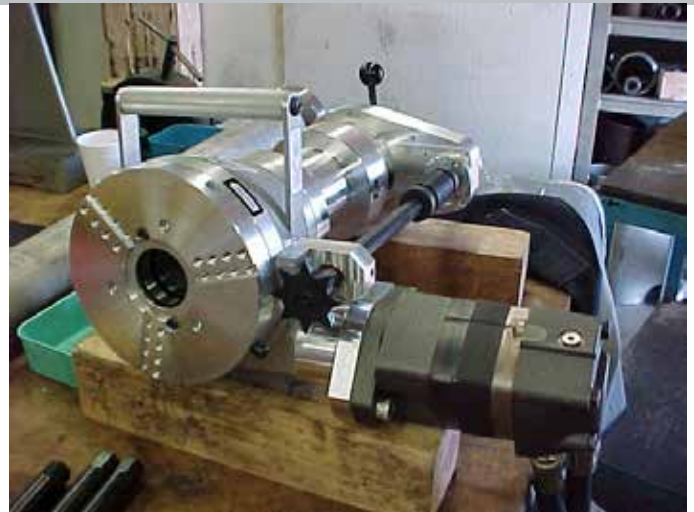
This custom 200 Series BEVELMASTER® ID mounted beveler features a hydraulic drive that is serving dual duty, providing drive power for the cutting head as well as operating an auto-feed system.
