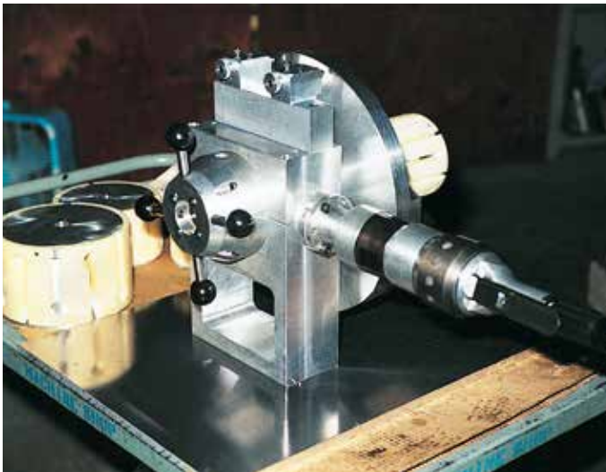
This ID mounted BEVELMASTER® has been custom engineered as a production, bench-mounted end-finishing machine for thin wall tubing with a special base plate and full support mandrel pads.
