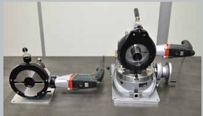
A great comparison shot of the standard (saddle clamping) Model 304, next to a custom 304 with Quick-Lock collet clamping and a special adjustable, offset bed for performing oblique cuts.
