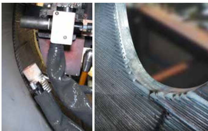
This custom welding fixture was designed to perform extremely accurate and rapid cladding on the ID bore of pipe to provide durable corrosion resistance intended for geothermal piping system repair.
