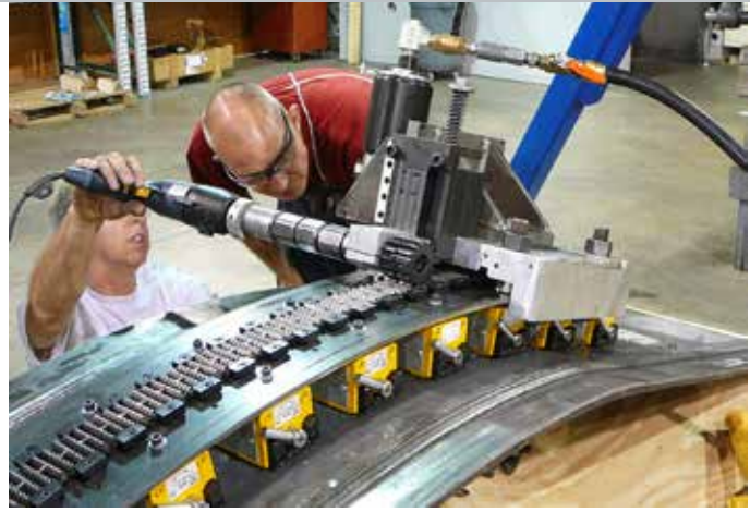
Sometimes it's not just the machine but the mounting system that must be custom manufactured. This special milling machine was designed to be able to conform to the curved side of a ship's hull.
