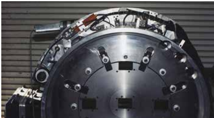
The nuclear industry demands that a wide variety of contingency equipment be kept on site to address any eventuality. This is a custom Omega Seal cutter with video cameras designed for remote operation.
