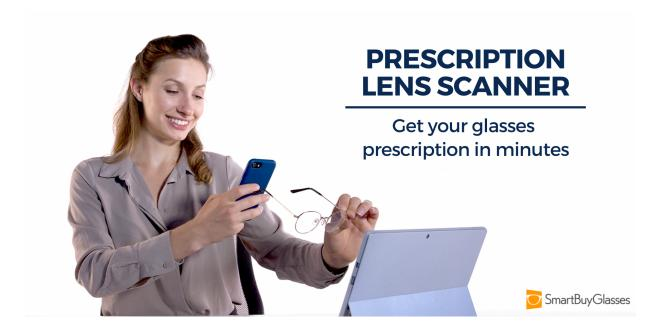
Not only is the Lens Scanner simple to use, but it also ensures precise prescription measurements. The readings are of the standard range of deviation used at in-person appointments and include the industry-standard range of +/- 0.25 diopters. The pupillary distance (PD) measurement is also within a +/- 1 mm of accuracy.
