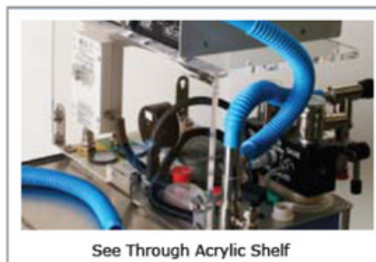
Waste Gas Tee connects APL Valve and Ventilator to Waste Anesthesia Gas Scavenging Manifold.
